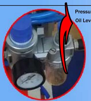
**Pressure oil chamber conditioner( No need to maintance-Easy To Use Pneumatic System)** Oil Level 0,2 - between 0,5 cm is suitable for pressure
