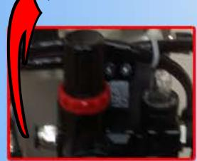
Step -2 You can adjust with allen key on die adapter hole bolt accordig to your dies height
